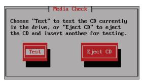
Pressing *Enter* with the **Test** button highlighted begins the test, which shows a progress bar. We need not worry about it referring to a **CentOS-4 i386 DVD**; this is due to the fact that TrixBox is derived from CentOS, which has a DVD version.
