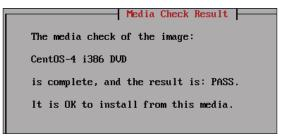
This means that we had no errors in the CD-burning process and that we have a valid CD to install from. Since the TrixBox installation is automated and requires little user input, the most common errors are due to the CD-ROM being burned with errors. If we see anything other than the preceding screenshot, or if it indicates a **FAIL**, we should burn the CD again and ensure our burning software verifies that the burn was successful.
